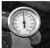
**Compost Thermometer** Stainless steel body and 19" probe, scaled from 0 to 220 in °F.
